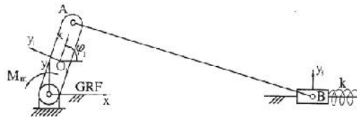
Figure 3. Schematic representation of slider-crank mechanism with dynamic elements
